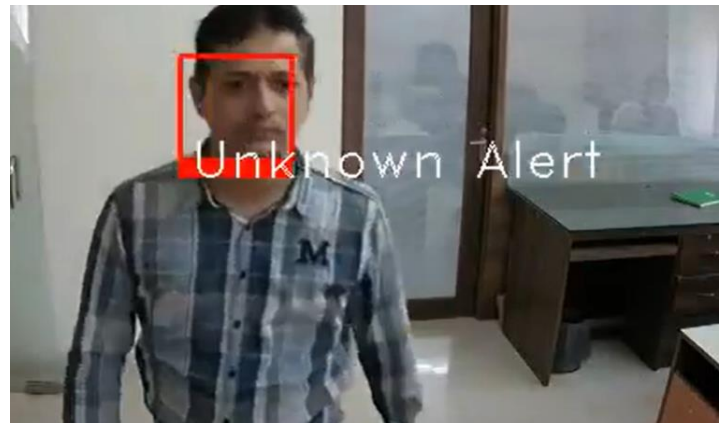
Fig 5: Unknown face detection using Python OpenCV
