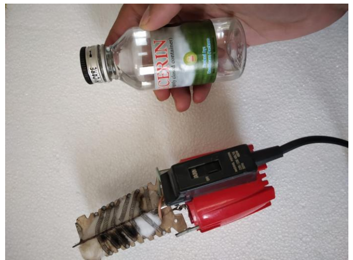
Fig 3: Fog Canon with Glycerol Solution
